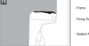
Coat the prime coat for original cement for 1 layer, and cover again by Acrylic Paint for at least 2 layers.
