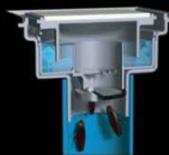
Water in the trap helps prevent the odor while automatic trap primer closes to prevent unwanted odor and pest coming from the sewage pipe.
