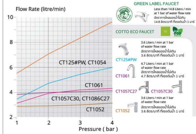
The graph shows a comparison of water rate at a different pressure of COTTO Eco Range
