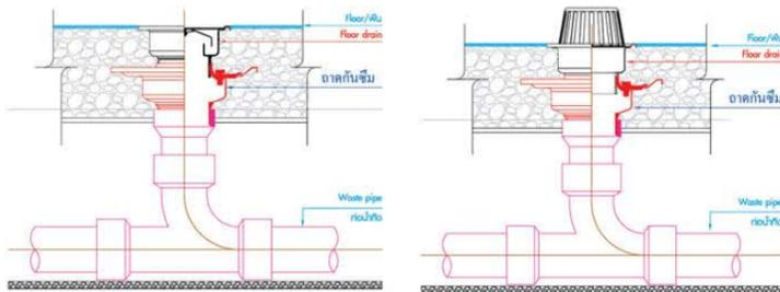
A schematic example of an Installation of anti-leak tray together with drain grates for both bathroom and balcony to prevent leakage from cracked surfaces or from eroded grouting around draining grates on to lower ceilings. With anti-leak tray, leaked water will be directed back to the drain.
