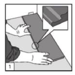
1. After check subflooring tolerance less than 3 mm. and dry, Must be installation of the EPE foam sheet with the thickness of 1 mm,
