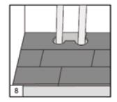
8. If there are any obstacles in the area which are higher than the installation areas, the SPC Floor with Click should be cut horizontally according to that obstacle. The additional space should be allowed for the expansion.
