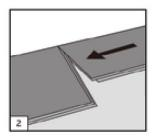
2. The Second plank, the first row- place this plank gently and tight to the short end of the first one.
