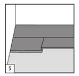
5. Starting the Second row the first plank should be a Half-length of piece (Or use the remaining plank from cutting the last plank of the first row to be the second row). Put a spacer against the wall and measure the last piece. If it is shorter than 30 cm. a new starter piece should be used. Insert the plank at an angle into the previous row and tap (on the long side) it in using a tapping block till flat.
