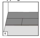
6. Fold the panel down in a single action movement with a slight press to the left to the short end of the previous panel. Again, using the tapping block tap it against the long end into the previous row. During the fold down, make sure the panels are tight against each other.
