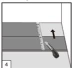
4. At the end of the first row, put a spacer 8mm-10mm to the wall and measure the length of the last plank to fit. The length of the cut SPC Floor should not be less than 30 cm.
