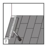
7. General distances between a long side ends. Minimum distance between a long side ends of the planks in parallel wall should not be less than 5 cm.
