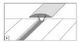
9. When installing of the products, please check the smoothness and the jointing between the planks. There should be no difference between each plank.
