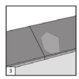
3. Fold the panel down in a single action movement. During the fold down, make sure the panels are tight against each other. Afterwards press down or slightly tap down at the short end just installed till it clicks. No major force is required.
